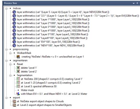
Figure 10: The ruleset used in eCognition. The children below the layer pre-processing node is specifically made for images from Google Earth Engine, since data is exported as scale ratios. Another image would not need this type of pre-processing.
