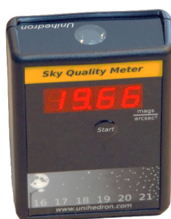
Figure 25: Sky Quality Meter – L (Narrow field of view, with Lens). This handheld device measures the brightness of the night sky in magnitude per square arcsec. (mag/arcsec 2 ). The SQM is produced by the Canadian company Unihedron ( http://unihedron.com/projects/sqm-l/ )
