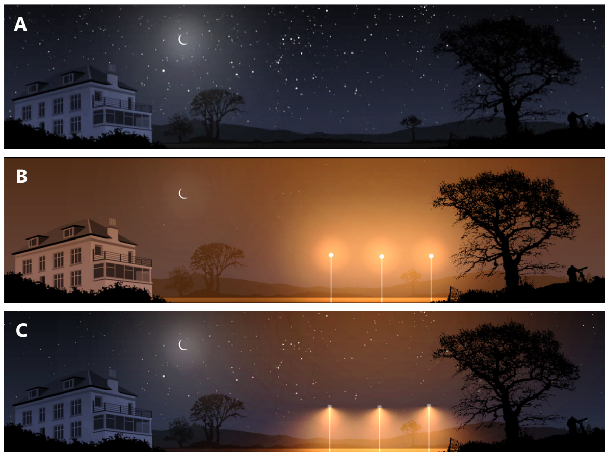
Figure 7: Visualization of the contribution of different types of light sources to light pollution. Image A shows a rural landscape without artificial lighting. In image B three unshielded luminaires with strong light emissions towards the sky are installed. The effect of the sodium-vapor lamps (creating orange light) is visible. Almost all stars have disappeared. The situation changes considerably in case the lamps are shielded towards the sky (image C).
