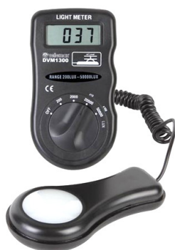
Figure 22: Light meter (Lux meter) used for the field measurements in this study: The device is composed of a sensor (lower part of the image) and a display of the measured light intensities (upper part of the image). The light meter captures the brightness of an environment. The unit of 'Lux' derives from the unit 'candela' which is another measurement of light intensity. (Historically, 1 candela was equal to the light intensity of one regular candle). The employed device is a handheld light meter from the Belgium producer 'Velleman', B-Gavere' (type: 'DVM1300'). ( https://www.velleman.eu/home/ ) :
