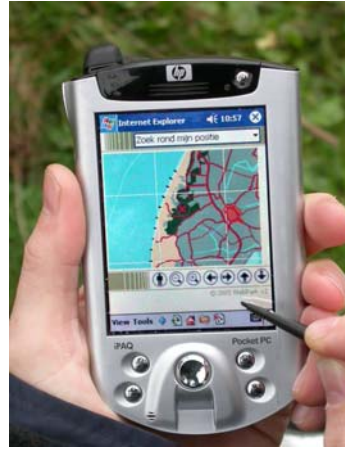
Fig. 4. Detail of the Mobile Information System. Topographic Map with user location (via GPS signal) for navigation purposes.
