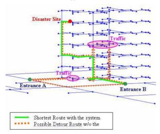
Figure 6: Navigation routes in a building (from Kwam and Lee, 2004)
