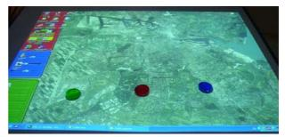
Figure 8: Geodan tangible user interface table (from Scotta et al, 2006)
